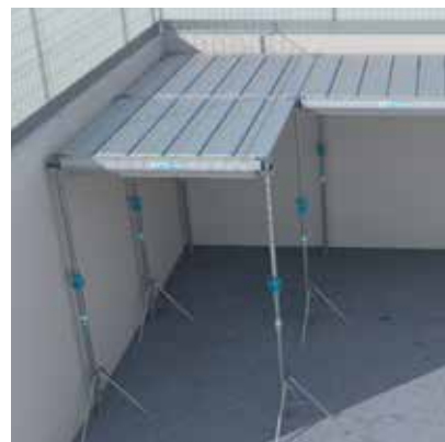
The extendable beams let you go near the cell edges
